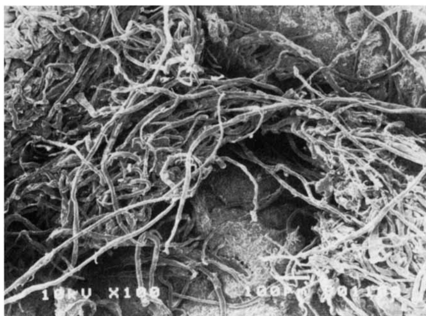
Figure 1 SEM photomicrographs of (a) untreated cellulose fibers and (b) Santoweb fibers.
