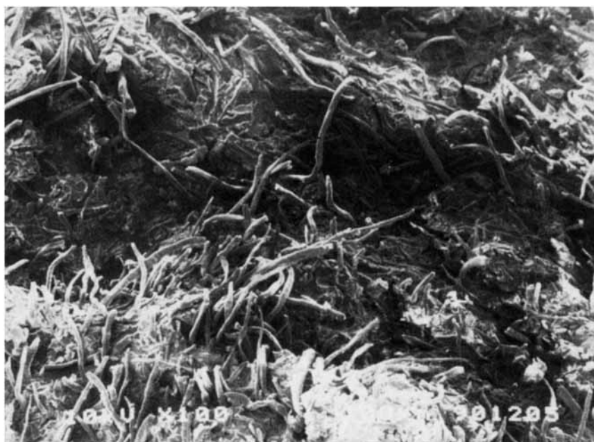
Figure 7 SEM micrographs of fracture surface: (a) 40% \alpha -cellulose/PS composite; (b) 40% Santoweb/PS composite.
